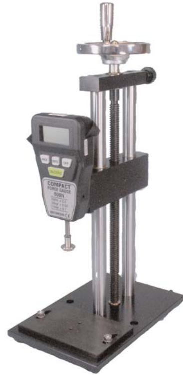
Shown with CFG digital force gage (Can also be supplied with BFG digital force gage)
